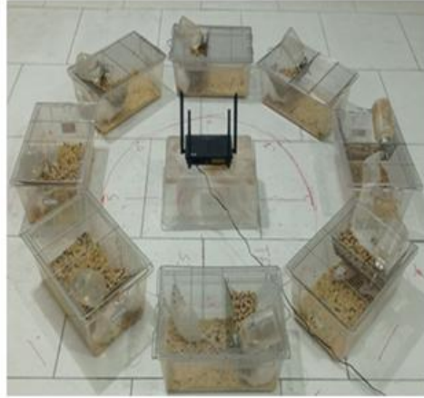
Figure 1. Setup of the electromagnetic exposure; wave: 2450MHz EMR by Wi-Fi router.
