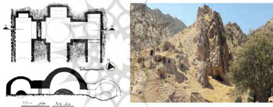
Figure 6. Plan and view of the Qalasangah Chahartaqi, (Nourallahi, 2005)
