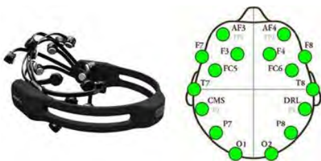
Fig. 2. Emotiv EPOC+ headset and its 16 sensors
