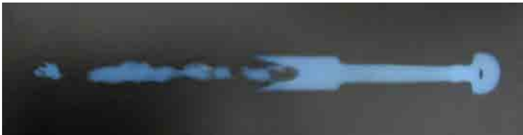
Fig. 5: The radiographic image of the object, with a potential difference of 100 kV and a current intensity of 50 mA (Original images: Soraya Mohammadi).
