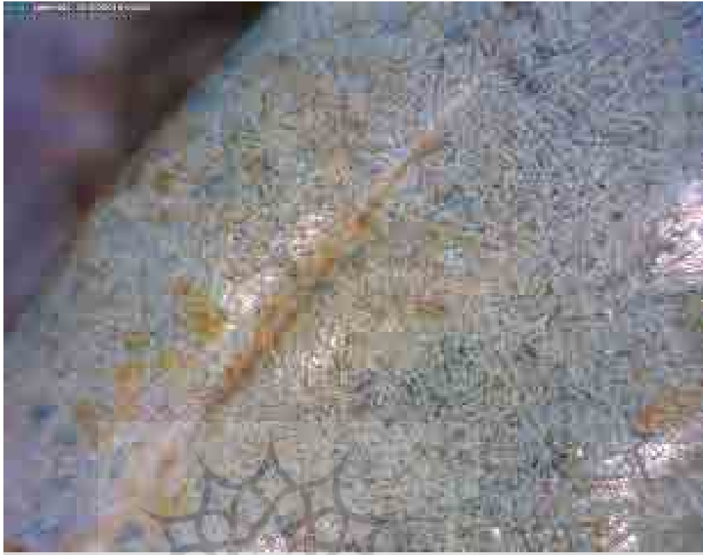
Fig. 6: Specific dendritic structure in the outer part of the end of the handle (Original images: Soraya Mohammadi).
