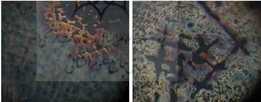
Fig. 7: (A)- Dendritic structure, copper corrosion in cored dendrites and inclusions with 200 x magnification – (B) - Dendritic structure and copper corrosion in cored dendrites, with 100 x magnification (Original images: Soraya Mohammadi).
