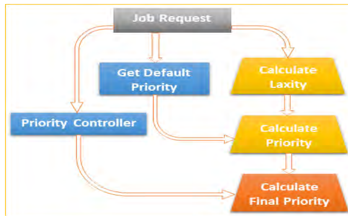
Figure 2. Priority calculation system with a control mechanism
