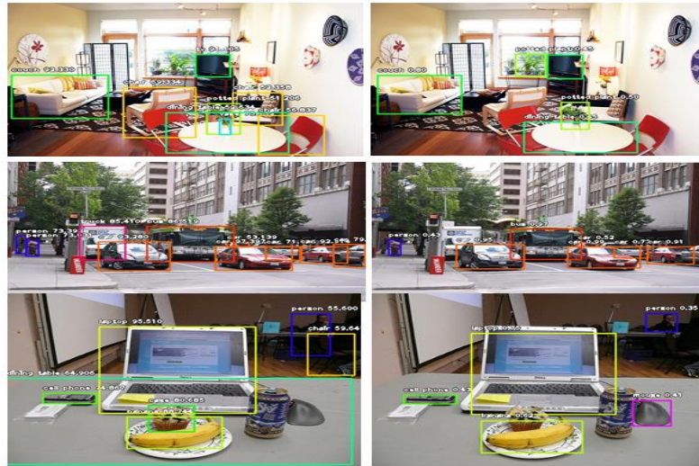
Figure 10. Object detection using ResNet 50 (left) and TinyYoloV3 (right)
