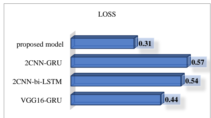
Fig. 6. Comparison of the loss for the proposed method with VGG16-GRU, 2CNN-bi-LSTM, and 2CNN-GRU methods on the MPerSocial dataset.
