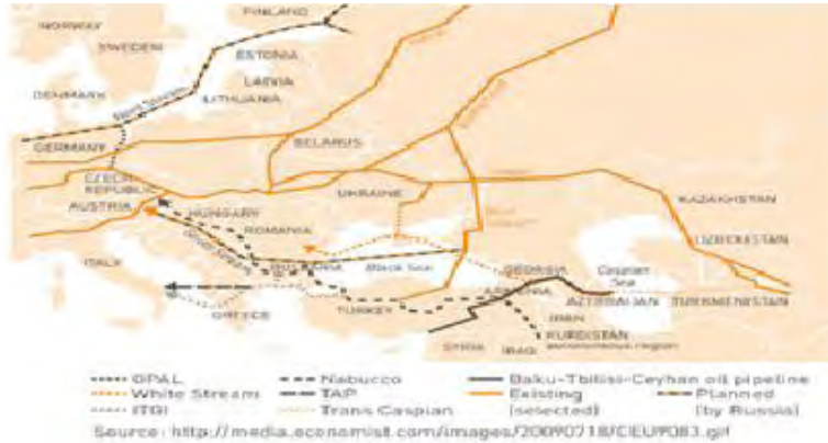
Figure 17. Available gas transmission pipelines feeding the EU
