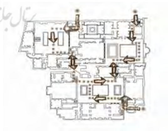
Fig.2: The rotational circulation plan in the House of Imam Jome'eh in Isfahan
