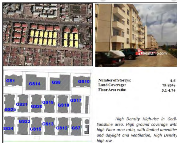
Fig. 16: High density high-rise with High BAR built-form pattern, no adequate spaces for amenities, parking etc. (Gerji-sunshine)
