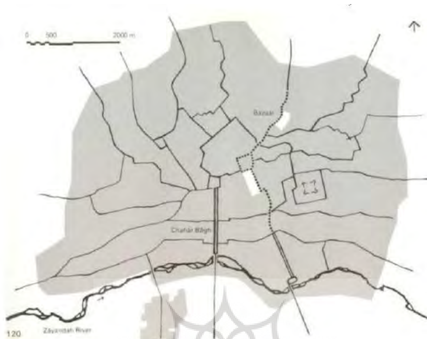
Fig.6: Schematic map of Isfahan's water channel (Madi) system, the Maddies made an organic design in the city (Ardalan & Bakhtiar, 1973)
