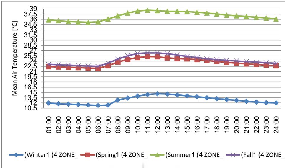
Fig.9: The thermal behavior comparison of five-door section in northwest orientation in the first day of different seasons
