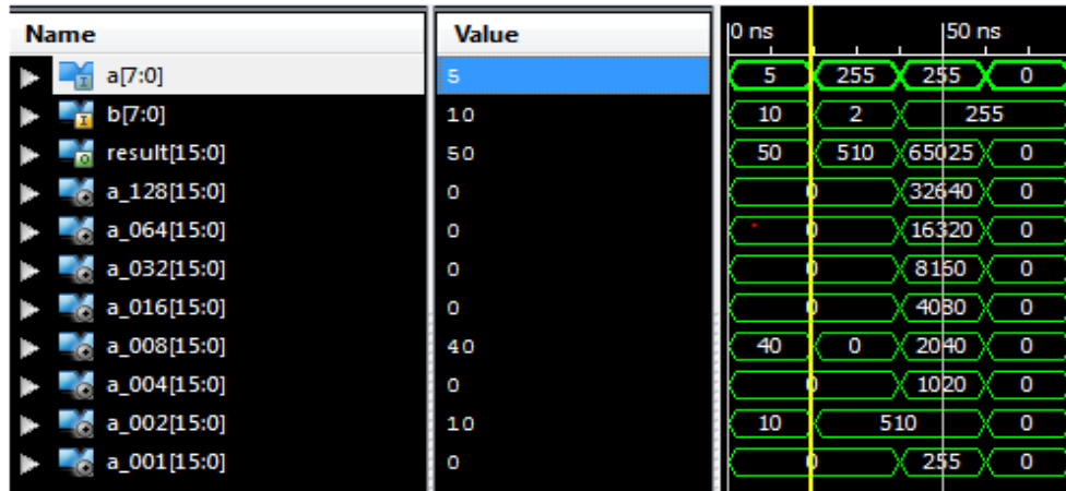
Figure 21. Simulation of the multiplication block under ISIM
