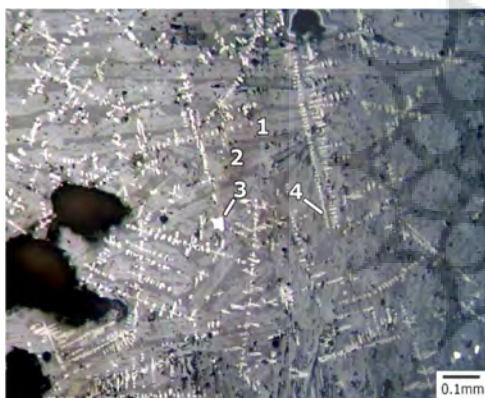
Fig.12. Microscopic View of the Slag in Fig.8—Dendrites of the Original Iron Oxide (4) Cutting the Elongated Fayalite Crystals (1) and Dark Glassy Background. Note the Almost Parallel Arrangement of the Iron Silicate Crystals along the Direction of the Primary Melt Flow
