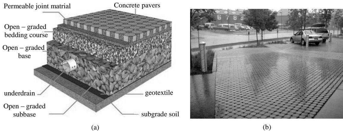
Fig.10. (a) Components of permeable pavement; permeable pavement
