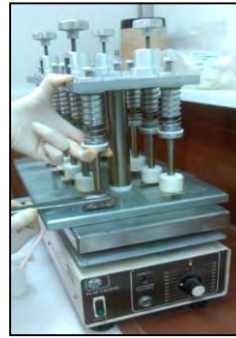
Fig; 8: Slide Chip coated with epoxy on the top of frosted slide put it on the flat heaters to penetrate resin and more connect the slide and chip to remove the bubble
