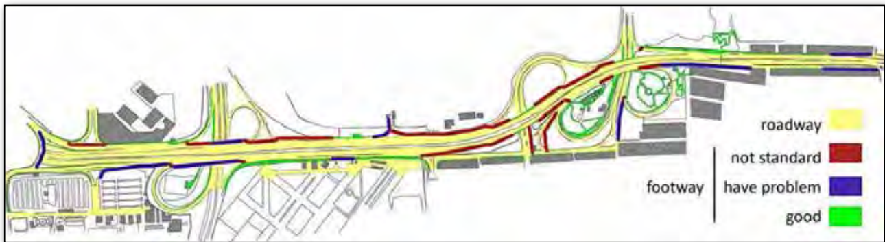
Fig. 13. Existing footways quality assessment along studied area corridor. Source: authors.
