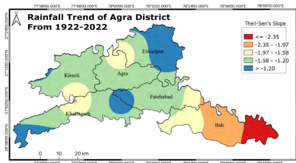
Fig 7. Rainfall trend of Agra district for all the data points calculated using the Theil-Sen's Slope
