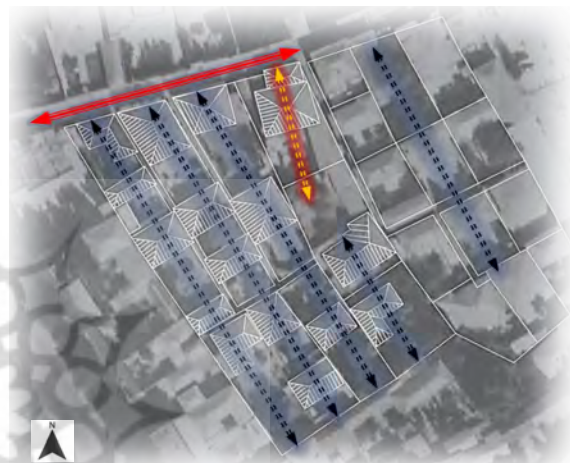
Fig.8. The building's orientation was primarily affected by the adjacent terrain and then it had natural light
