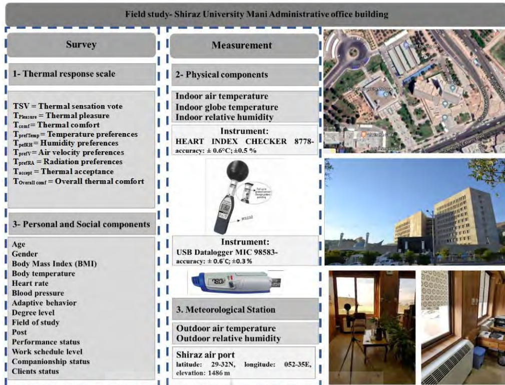
Fig.1. Measured components & used instrument during field study
