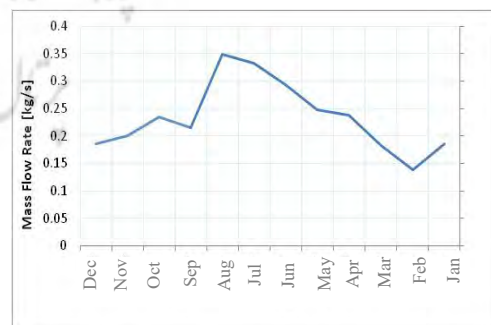
Fig.20. Total flow of solar chimney model two in one year
