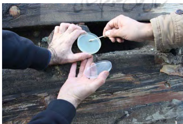
Fig. 6. A view of the sampling method of fungal and microbial agents from the hull of the ship (Authors, 2018).
