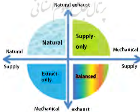
Fig.7: basic types of ventilation systems.
