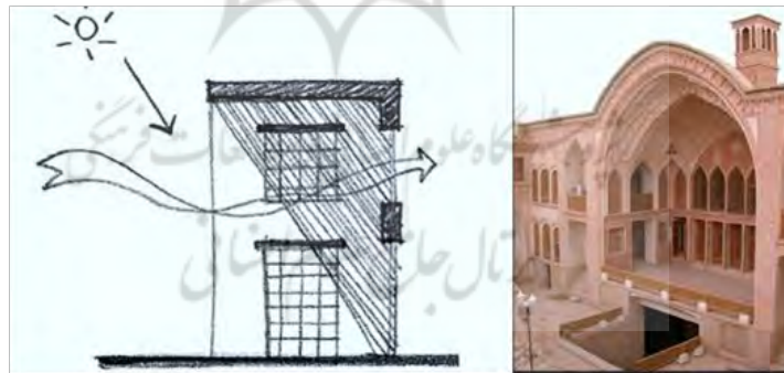
Fi g. 3: Porch as a shed in vernacular Iranian architecture (Source: Wong et al. 2008)
