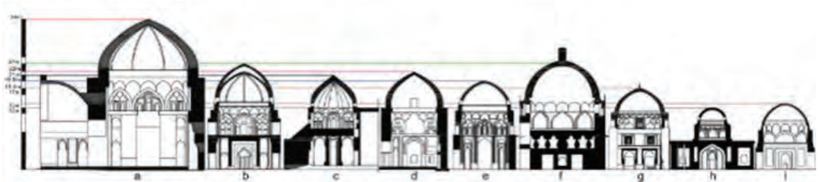
Fig. 9: Various dimensions of Seljuk's domed chambers in Central Iran in comparison with Northwest Iran caused by different technology used in the transition areas.
