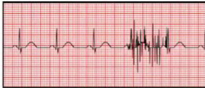
Figure 4. Electrocardiogram (ECG) signal with Electromyogram (EMG) noise reproduced from http://www.mauvila.com/ECG/ecg_artifact.htm
