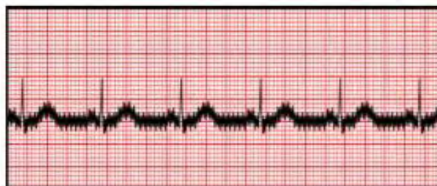
Figure 3. Electrocardiogram (ECG) signal with power line interference reproduced from http://www.mauvila.com/ECG/ecg_artifact.htm
