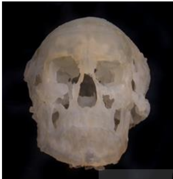
Fig. 13. Solid polymer model made by SLA machine (CAD/CAM)
