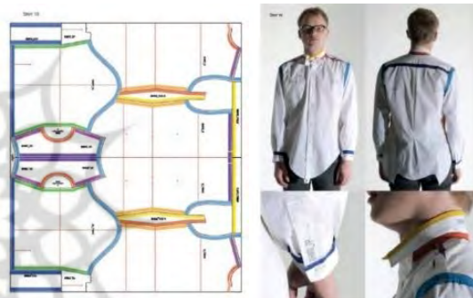
Figure 3. Men shirt with pattern and digital printing, display of direct relation between two-dimension pattern and three-dimension clothes (McQuillen, 2018)
