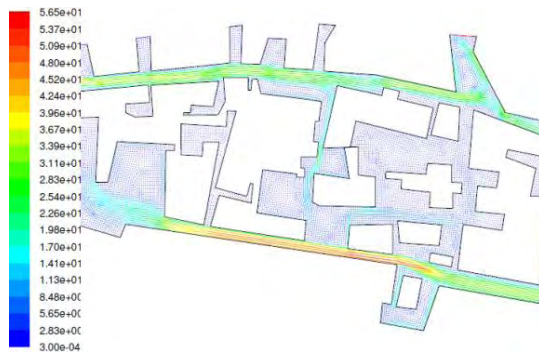
Fig. 5 Velocity vectors around the school
