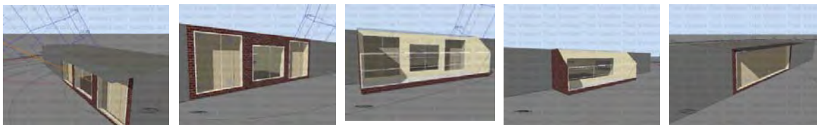
Fig. 5 Trombe wall with window and Shading
