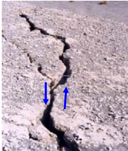
(Fig12): One of the fissures and fractures of the earth surface in silt deposits with easterly-westerly Direction lying to the west of Baravat and southeast of the Bam city
