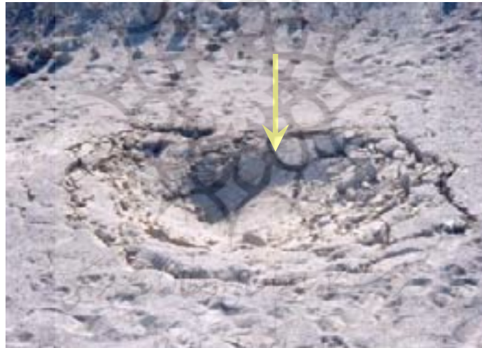
(Fig11): Sand deposits subsidence in the west of Baravat and southeast of the Bam city.
